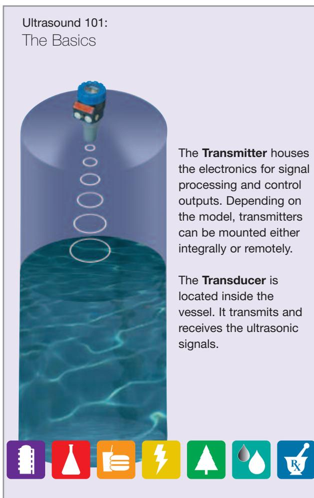
more dense, resulting in slower sound velocity. Since measurement is directly dependent on sound speed, it is necessary to compensate for temperature changes. All Magnetrol's EchoMaster® transducers include a temperature compensation circuit which continuously monitors the temperature at the sensor and compensates for variations over the full temperature range of the transducer.
